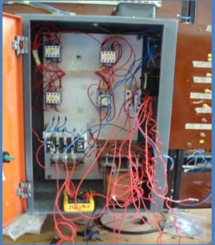
Seaman Truter did an assignment on an auto transformer panel which forms part of the normal trade test.
