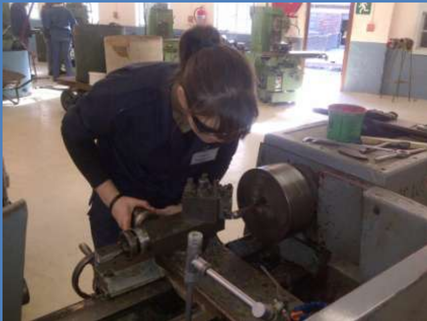
Seaman Bezuidenhout working on the lathe making the handle for the tack hammer.
